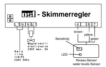
The sensor cable can be extended with a shielded four-conductor cable. The extension has to be carried out water-proof in order to avoid creeping current due to penetrating humidity. The shielding of the extension is to be connected with the shielding of the sensor cable (and with the green wire). The shielding must not be connected in the control unit.
